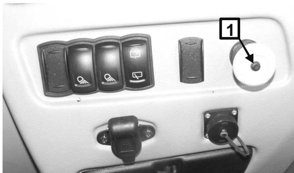
Figure 4-30 PTO activation switch on PRONAR tractors and method of engaging PTO drive. 1- rear PTO switch
