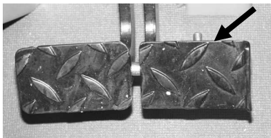
Figure 4-24 Catch locking working brake pedals.
