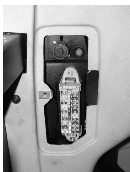
Figure 5-32 Location of set of fuses on left side of steering column. A- screw; B- cover
