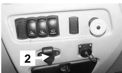
Figure 5-29 Connection 1 of electrical system and socket 2 for supply +12V 20A to additional receivers connected to tractor electrical systems.
