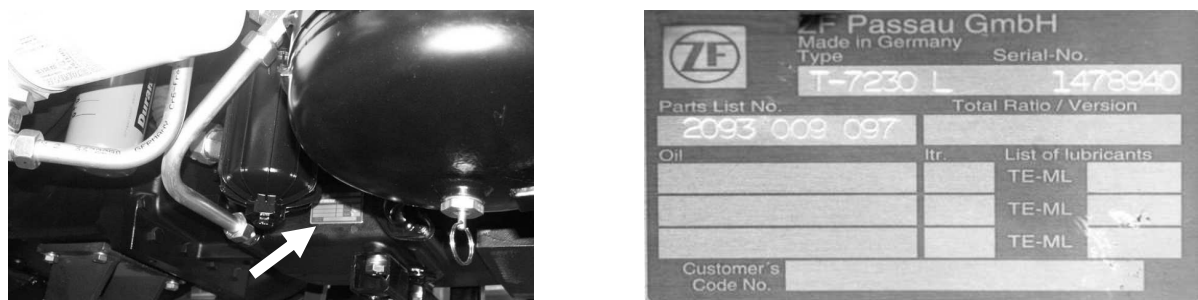
Figure 3-4 Location of transmission system plate (on right side of tractor on gearbox casing)
